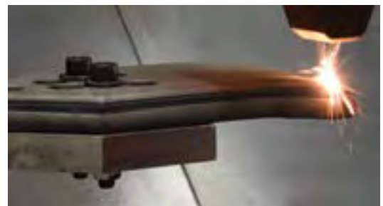
Laser cladding is robotically applied resulting in pinpoint accuracy
